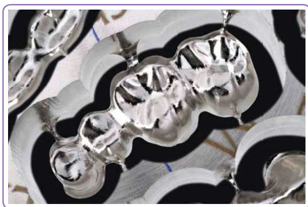
Very smooth and shiny surface (CoCr milled).
