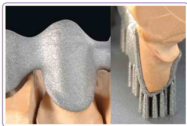
Excellent fit (CoCr SLM).
